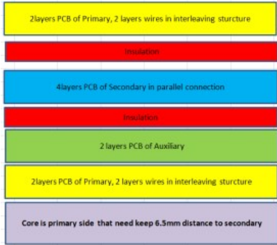
a) Transformer winding cross section
